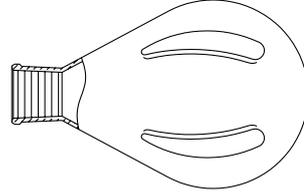
Special flask for drying powdery substances. The integrated baffles encourage thorough mixing and prevent crusting of the sample.
