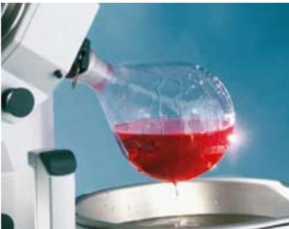
In the event of a power failure or a fault in the bath, the flask is automatically raised out of the heating bath to prevent over-heating of the product.
