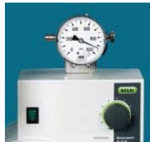
Setting of using a needle valve with simple display. For use in combination with vacuum Woulff bottle.
