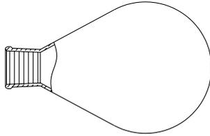
Pear-shaped evaporator flask, with standard joint
