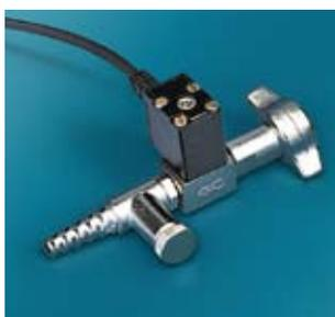
Helps to save water, as the cooling water feed does not have to be manually switched on and off. The vacuum controller opens the cooling water feed only during distillation.
