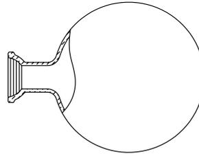
Round receiving flask with ball joint pan KS 35-20. With or without P+G coating.
