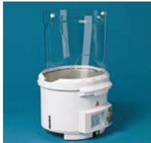
Effective protection against splashing or a possible flask breakage.
