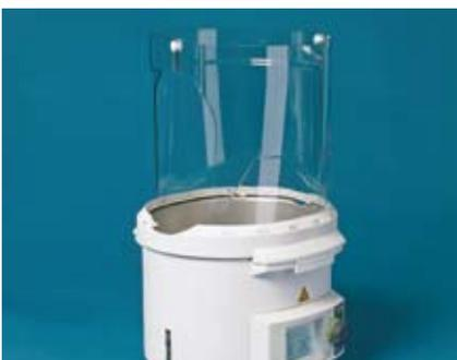
The transparent safety guard is ideally matched to the design of the heating bath and is easy to fit. This accessory provides effective protection for the user against splashing or a possible flask breakage.
